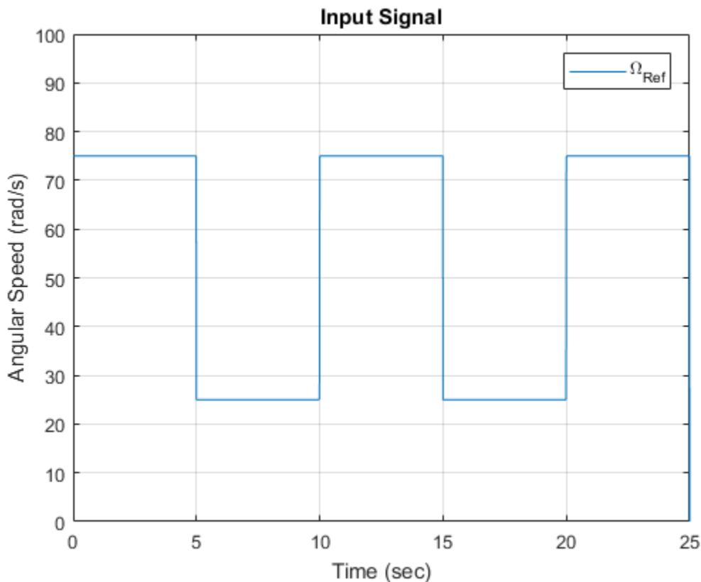
2. Value of the input voltage  $V = \text{Angular Speed}/28.5$
