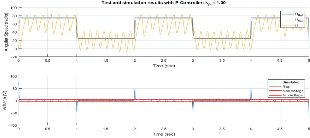
No, because the addition of the controller has introduced oscillation in the system output, which is not desired.
