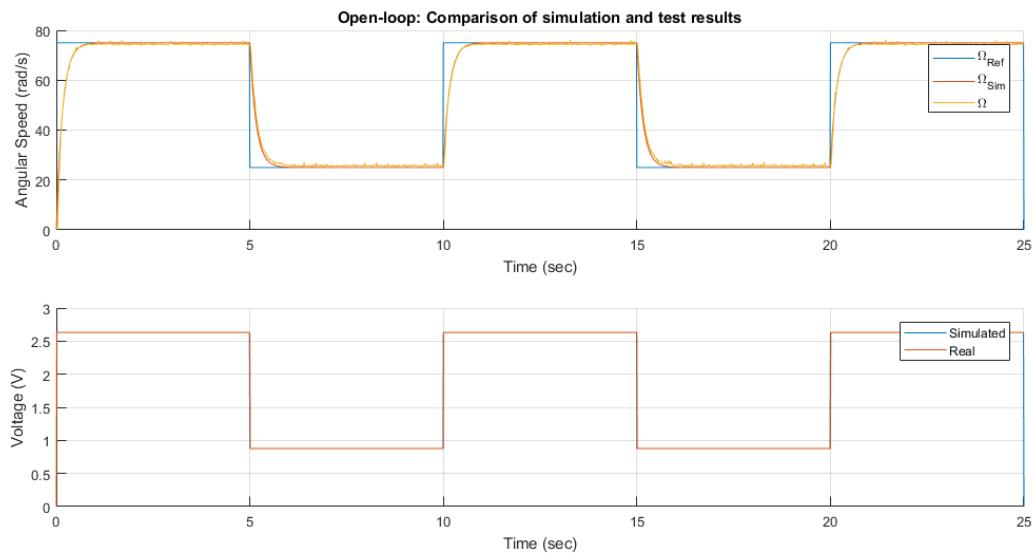
5. Outcome of the discussion: The proposed model  $H(s)$  describes the Qnet DC Motor with satisfactory. The model tracks the motor output, except for a difference in the rise time. If the frequency is five times bigger, the output would be more curved and the model will not be able to properly track the Qnet DC Motor.
