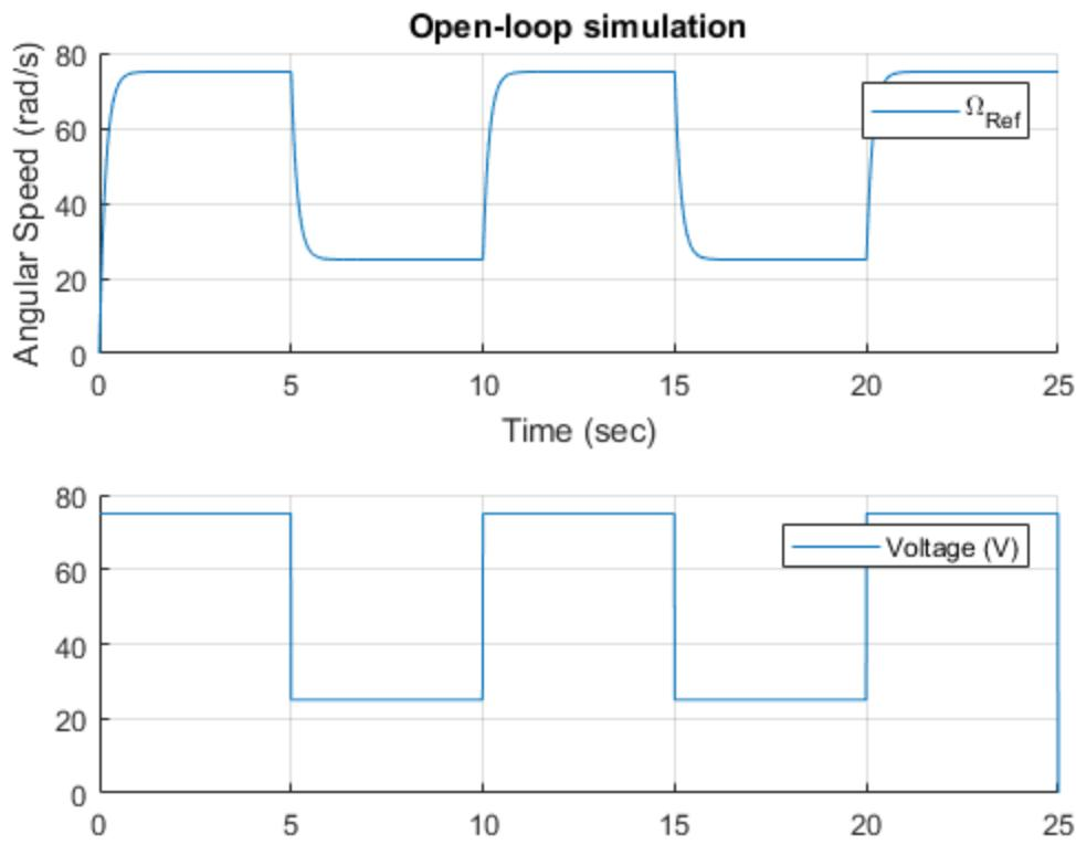
4. Response of the transfer function  $H(s)$ , superimposing the Qnet DC Motor and the simulation
